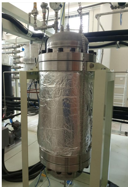
Fig. 10: Extraction vessel of pilot scale CXLE at the University of Dar es Salaam, Tanzania
